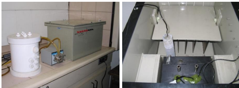
Electrochemical conversion cell for H 2 S removal
