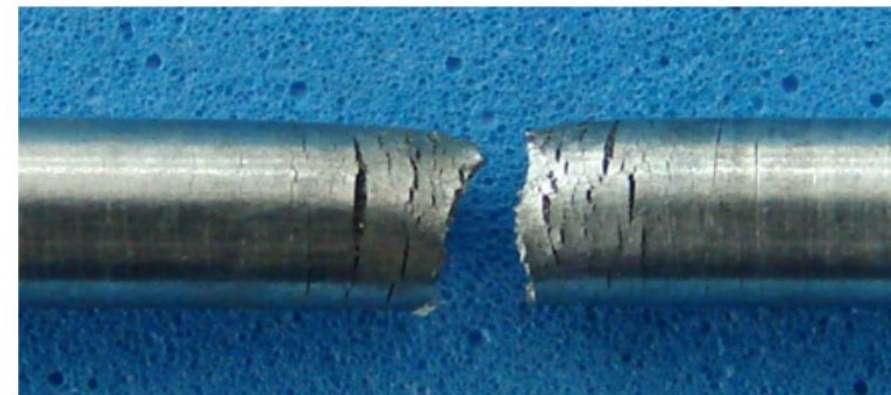
Fig.: SCC on a Martensitic Stainless Steel
