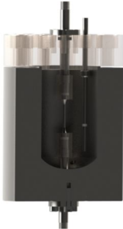
S_{L-H_2} (H_2) Autoclave System up to 70MPa
